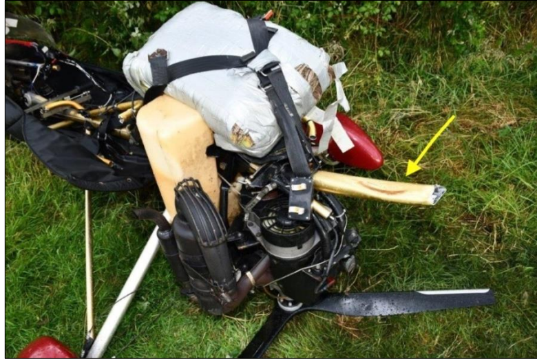
Photo No. 4: Vertical support post with evidence of buckling and fracture
