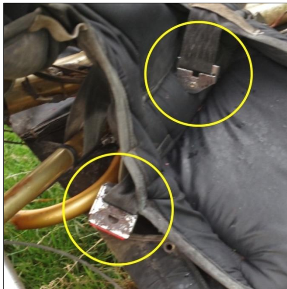
Photo No. 6: Front seat lap-belt ends (indicated) exhibited significant corrosion of the latching mechanism
