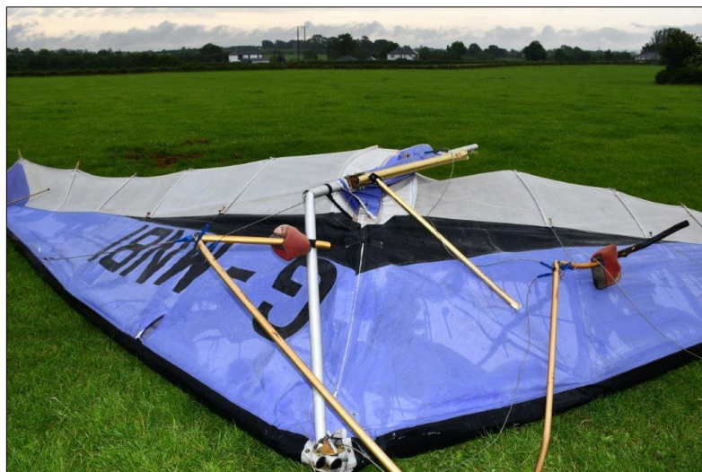
Photo No. 3: Under-side of wing, showing fracture of control-frame components
